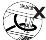
▲ Always route the gas hose away from the oven. The hose must not touch the oven body.
