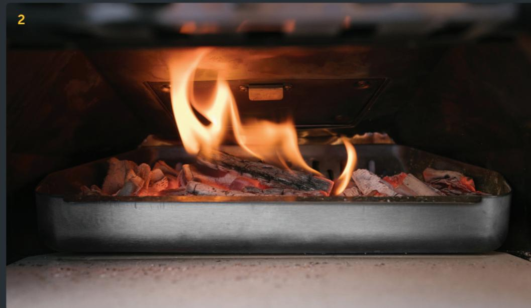
Ooni Karu 16 is not ready to cook a 60-second pizza when the fuel tray looks like this. If this is your scenario, gradually build up a flame using smaller pieces of kindling, allowing for good airflow through the grate. Always give new fuel enough time to burn properly before you start cooking.
