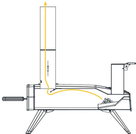
**Open chimney baffle** : Increases the draw of air through the oven, creating more powerful flames and an increased heat.
