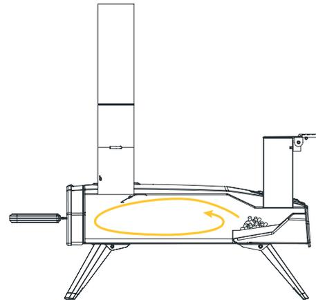
**Closed chimney baffle** : Reduces the draw of air and airflow for a smokier effect and a lower heat. Do not completely close the baffle for extended periods as this can cause the pellets to swell and jam.
