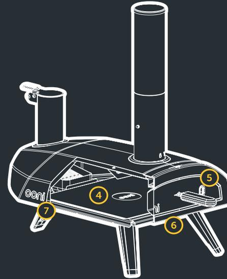
4. Pizza Stone baking board custom-made from cordierite stone for optimized heat retention and the perfect pizza base.
