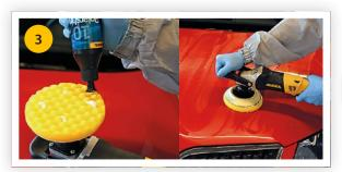
Apply 3–4 drops of polishing compound on the lambswool pad. Polish at 800–1,400 rpm. Polish until the final gloss has been achieved. Clean the surface from polishing compound residues before the next step.
