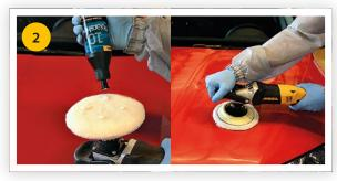
Apply 3–4 drops of polishing compound on the lambswool pad. Polish at 800–1,400 rpm. Polish until the washing marks and scratches have been minimised on the surface. Work with a small area at a time, about 40 x 40 cm. Repeat the procedure until the all surfaces have been checked. Clean the surface from polishing compound residues before the next step.
