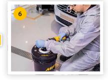
Lift the polisher and spin the pad dry at 1,500 – 2,000 rpm.
