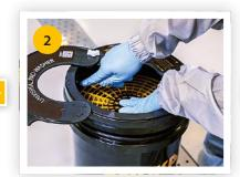
Press down the washing grid and fill the bucket with water until it is slightly above the washing grid.
