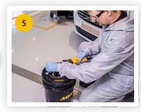
Press down the polisher against the grid and runt the polisher at approximately 800 – 1,200 rpm.
