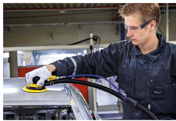
» Mirka® DEROS or Mirka® PROS with Abranet products or Q.Silver Ace P320–P400. Sanding on larger areas.
