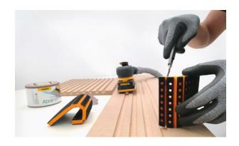
Groove Medium and Soft interfaces have 12 pre-cut segments of 12.5 mm. Depending on the width of the mouldings for sanding, users can simply detach the segments required from the interface, apply them to the plate of the Mirka® DEOS 343 CV 75x100 mm electric sander and add Abranet® or Abranet® Ace net abrasive strips.
