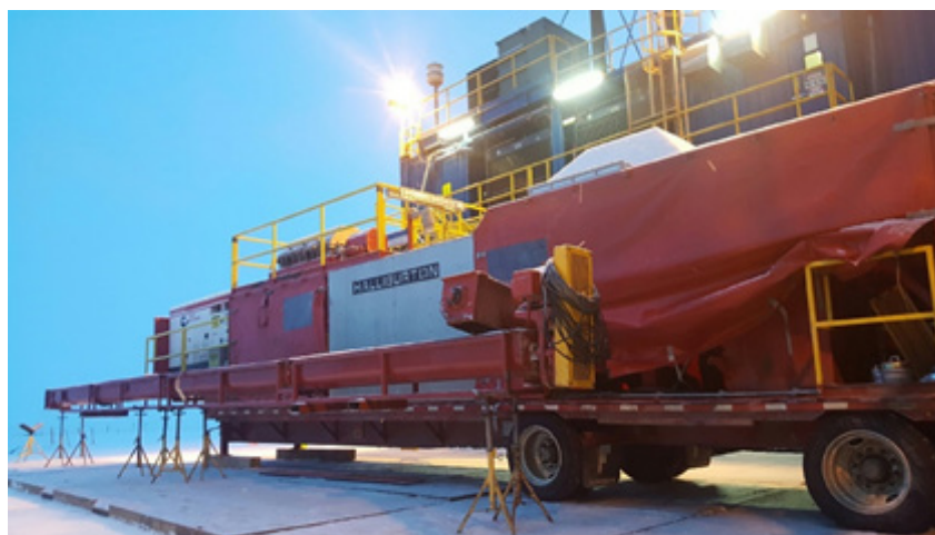
Trailer-mounted MVCD unit pulled up alongside of rig prior to drilling.
