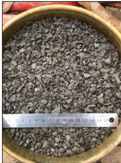
Cuttings from the shaker clearly showing preserved condition with cutter marks on surfaces.
