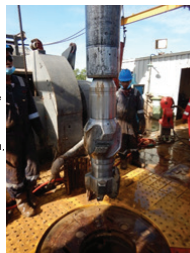
Bottomhole assembly on surface at Suban Field.
