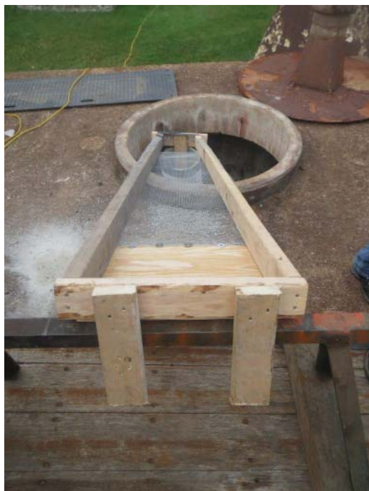
Screen Trough design for separation of "fines" from \frac{3}{4} " HOLEPLUG®
