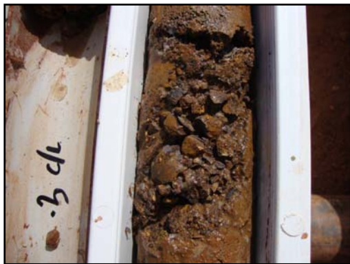
FUSE-IT™ liquid LCM bonding loose friable formation together
