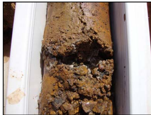
FUSE-IT™ liquid LCM bonding loose friable formation together
