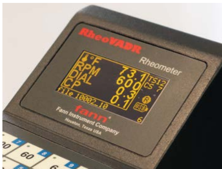
Figure 5-6 Test in Progress (API Test Mode)
