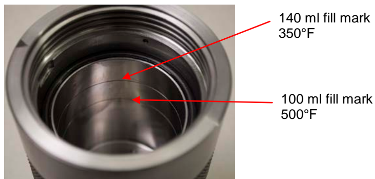
Figure 4-2 Cell showing fill marks inside
