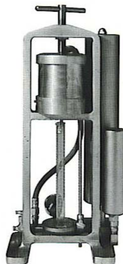
Hydraulic Dead Weight Assembly shown attached to Series 300 LPLT Filter Press
