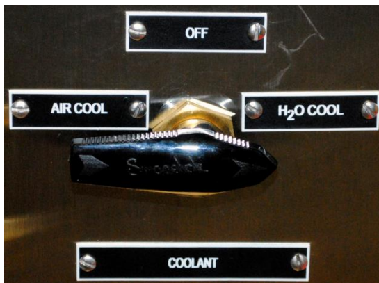
Figure 5-6 Coolant Valve open for water flow
