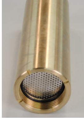
Figure 5-3 Screen and O-ring in Sample Chamber
