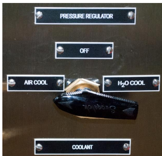
Figure 5-8 Coolant Valve open for air flow
