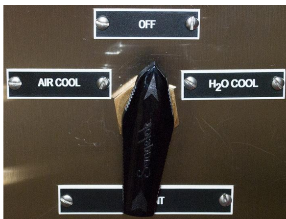
Figure 5-7 Coolant Valve in off position
