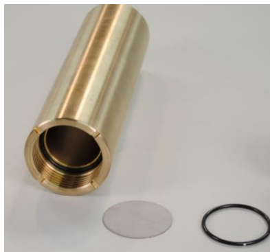
Figure 5-2 Brass Spacer and O-ring in Sample Chamber
