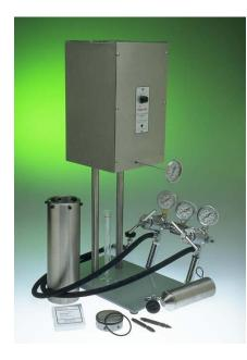
**500 ml HPHT Filter Press** units can be pressurized to 1800 psig on the cell and 750 psig on the back pressure receiver. Maximum operating temperature is 500°F. For operation above 400°F, the filter paper should be backed with a glass fiber filter, or a stainless steel filter.
