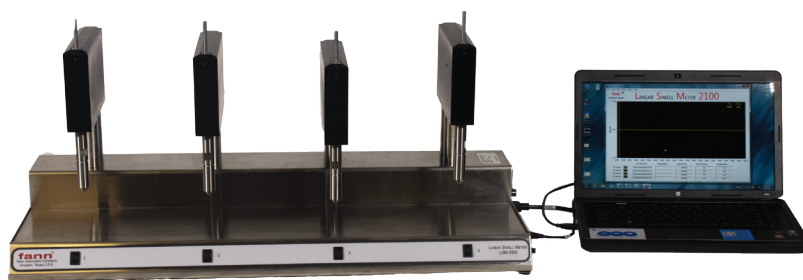
Model 2100 Linear Swell Meter
