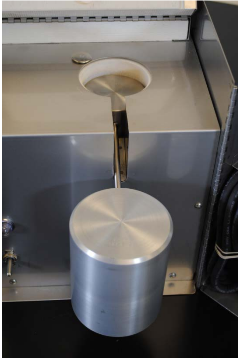
Figure 4-1 Retort Assembly in Heating Compartment
