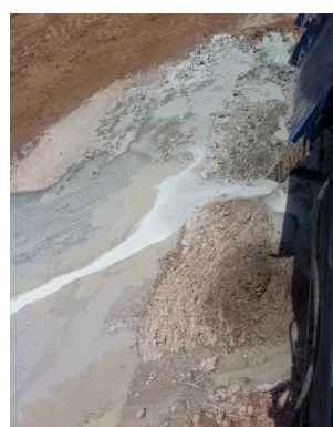
Figure 9: Spoils of the hard gray shale and sand portions of the bore, first 1000 ft.
