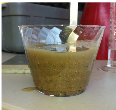
Figure 7b- Stirred in sand remained suspended for several hours without agitation.
