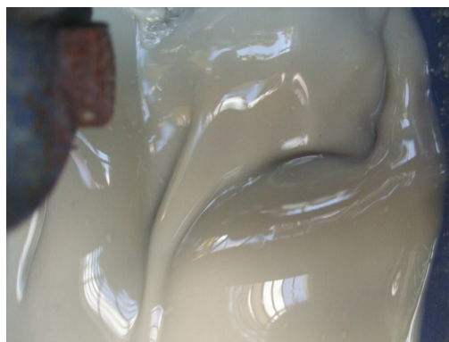
Figure 2: After addition of QUIK-TROL GOLD polymer and NO-SAG suspension enhancer the viscosity of the fluid visibly increases.
