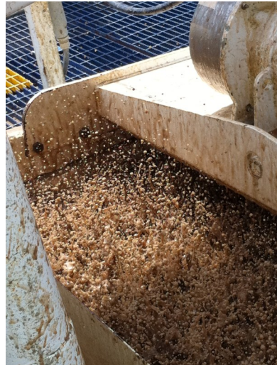
Figure 4: Shakers removing sand from returning fluid. The first 300 ft. were sand and gravel.
