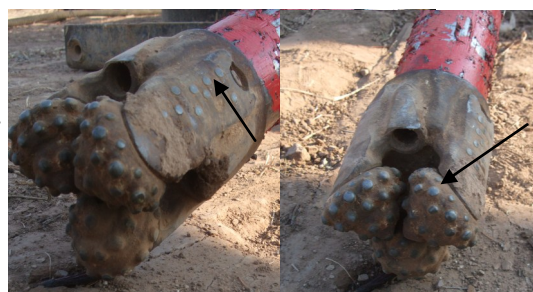
Figure 6— worn teeth on bit, balled with clay.
