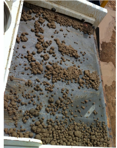
Figure 5: Sands removed from fluid by shaker screens.
