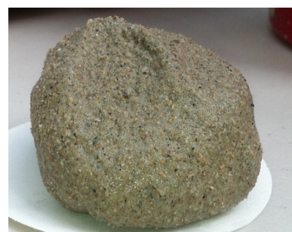
Figure 8b- Sands removed from circulated fluid with shaker screens on solids control equipment.
