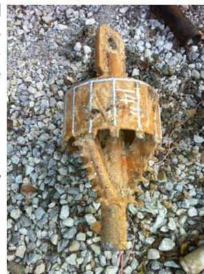
Figure 10- 14 inch hole opener reamer
