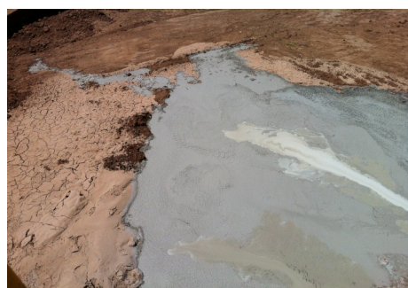
Figure 9: Spoils of the hard gray shale and sand portions of the bore, first 1000 ft.
