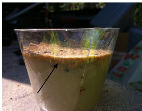
Figure 7a- Suspension demonstration. 1 cup of drilling fluid with NO-SAG enhancer with a handful of sand on top. Sand remained on top of the fluid until stirred in.
