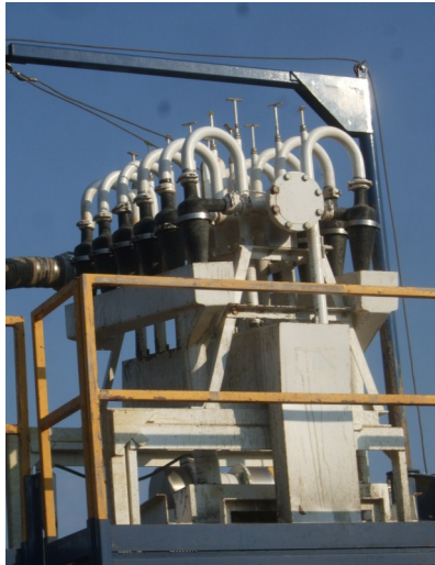
Figure 3: Tri-Flo solids control De-sander Cones
