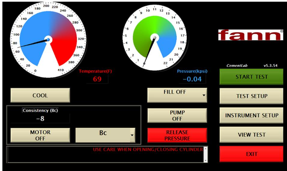
The main menu is starting point for the instrument. From here users may start new tests, set up test parameters, setup instrument parameters, or view an old test. Also located on the main menu is the reading for current temperature, consistency, and pressure. On the right side of the screen, the version software that is currently installed on the instrument is displayed. In the screenshot above, the version is 5.3.53.
