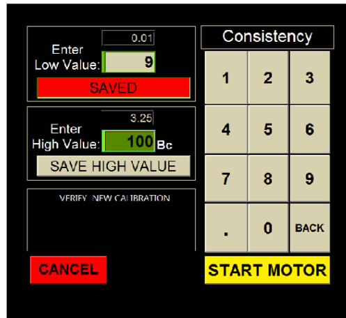
9. By removing weight from the hanger it is possible to verify the CALIBRATED VALUE as shown below. If the values are correct, calibration is complete. If the values are incorrect, repeat steps making adjustments to potentiometer mechanism as required. Refer to Table 5-1 for weight to Bc conversions for pot-mech.
