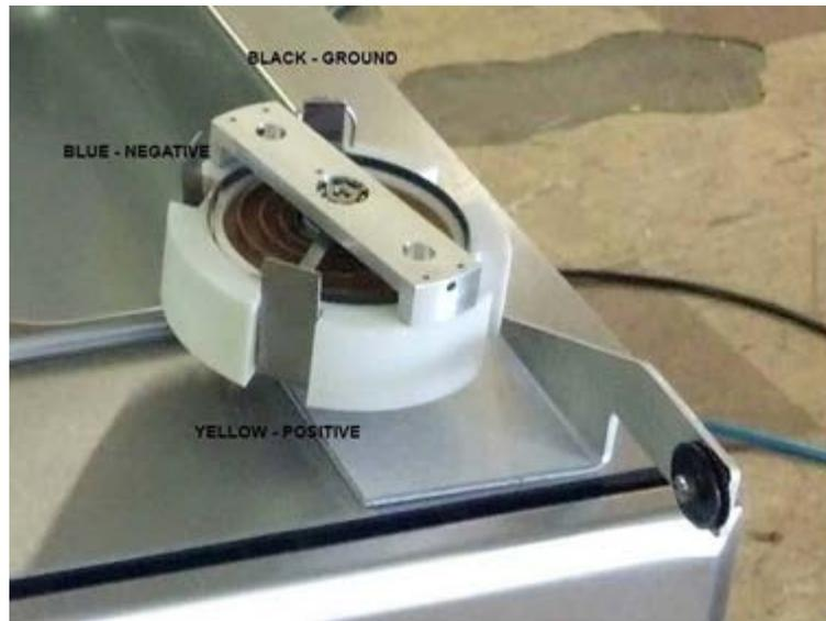
**Figure 5-1 Alligator clips attached to potentiometer mechanism springs**
