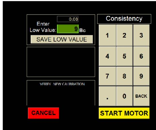
8. Place 400g of weights on the weight hanger. This is the equivalent of 100 Bearden Units of Consistency (Bc). On the touchscreen in the box labeled HIGH DATA POINT input 100 on the touchpad. Select SAVE HIGH VALUE. It may be necessary to tap the calibrator base to loosen any wound tension in the spring while in this screen.
