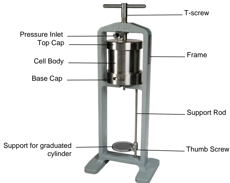
Figure 3-1 Basic Filter Press Assembly
