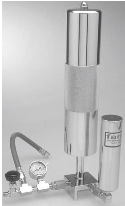
Figure 10-6 Dead-Weight Hydraulic Assembly
