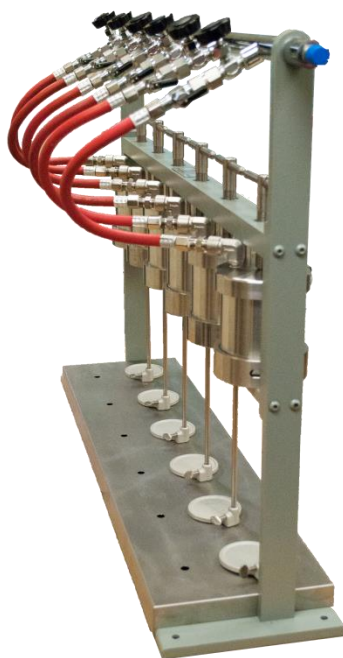
Figure 10-9 Six Unit Filter Press w/Manifold
