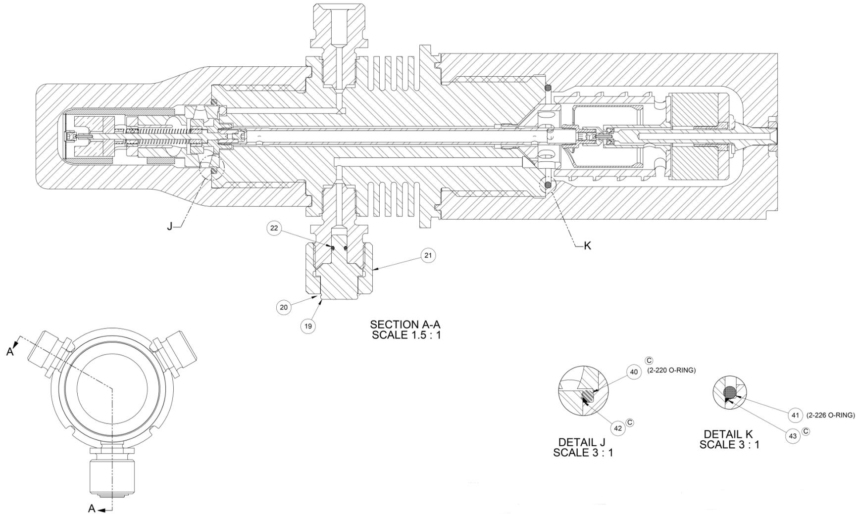
Figure 9-14 iX77 Cell Assembly
