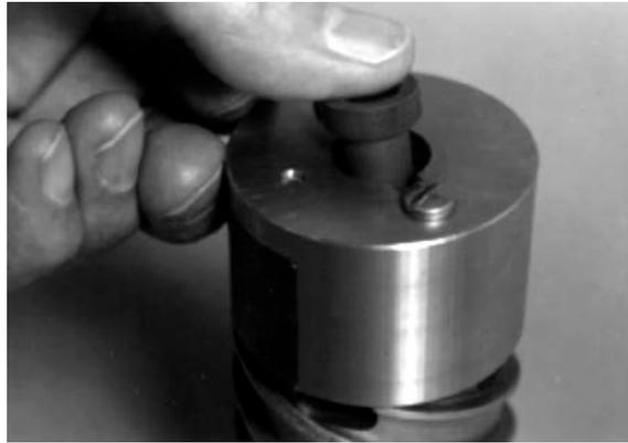
Figure 5-55 Pushing the rotor bushing into position
