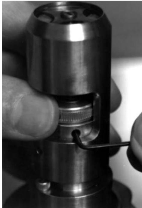
**Figure 5-59** Adjusting the zeroing sleeve
