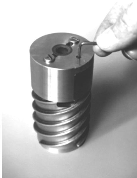
Figure 5-56 Locking the drive magnet
