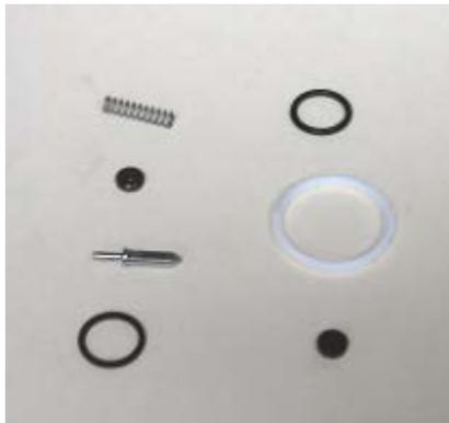
**Figure 7-18 Valve Parts**
