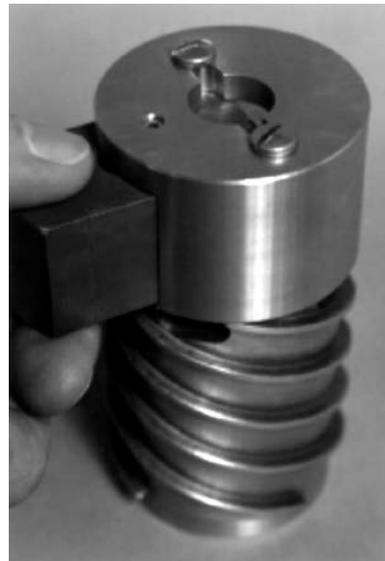
**Figure 5-54** Placing the drive magnet into position
