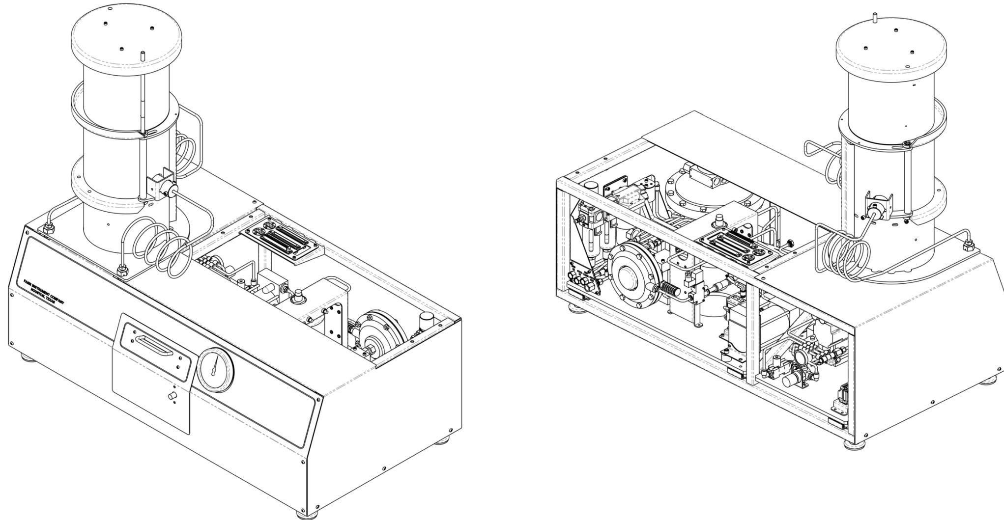
Figure 9-1 iX77 Mechanical Assembly, Front & Back View
