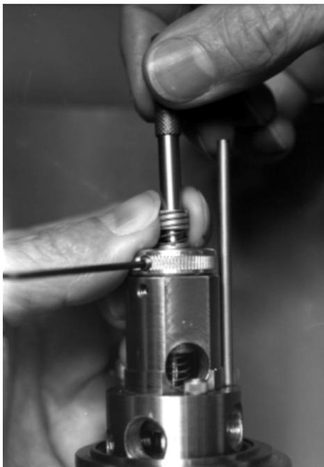
**Figure 5-63** Adjusting the torsion spring length
