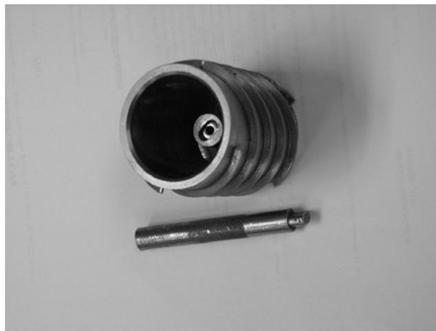
**Figure 5-49 Rotor and bearing removal tool**
