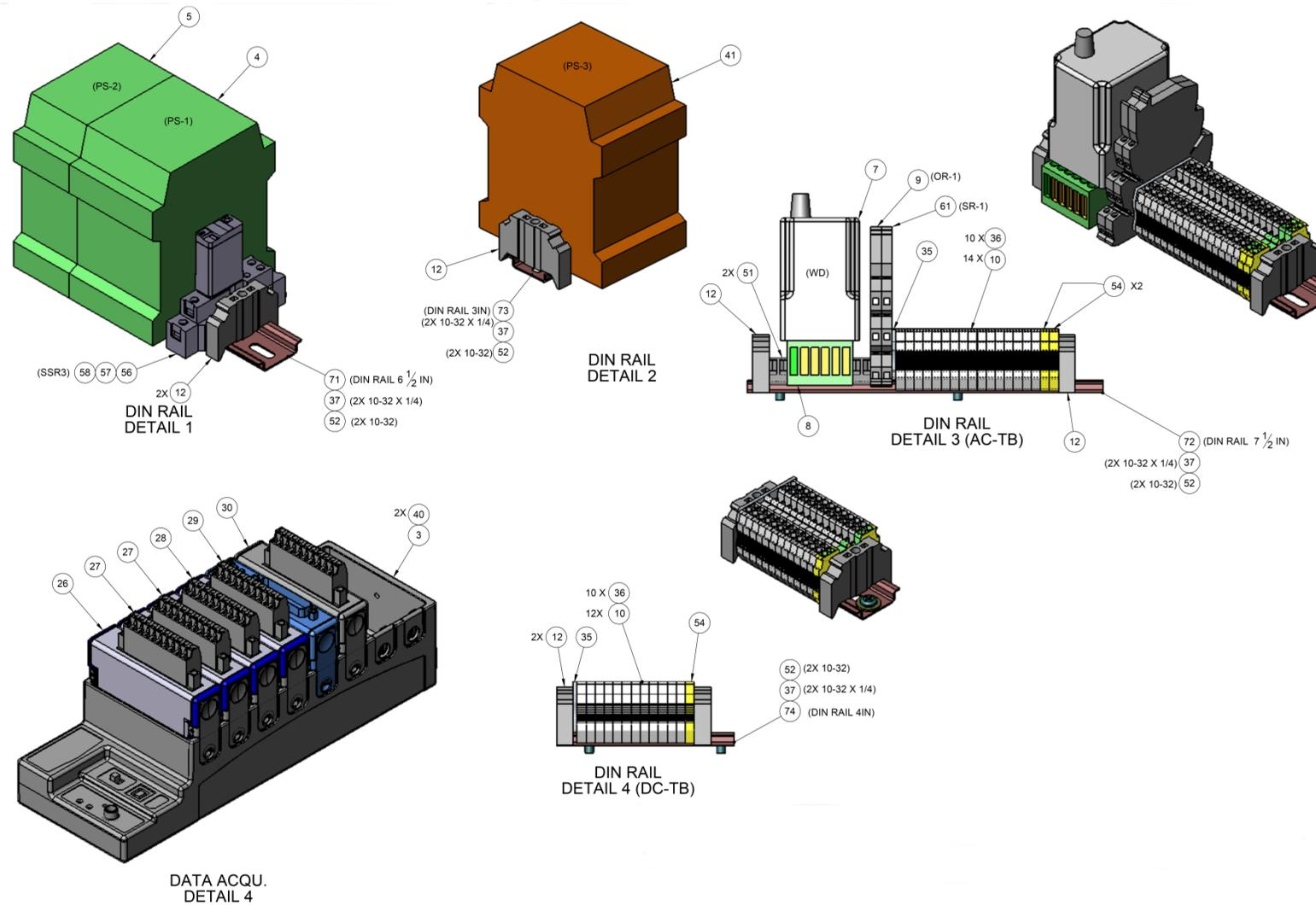
Figure 9-10 iX77 Electrical Assembly, Din Rail Components
