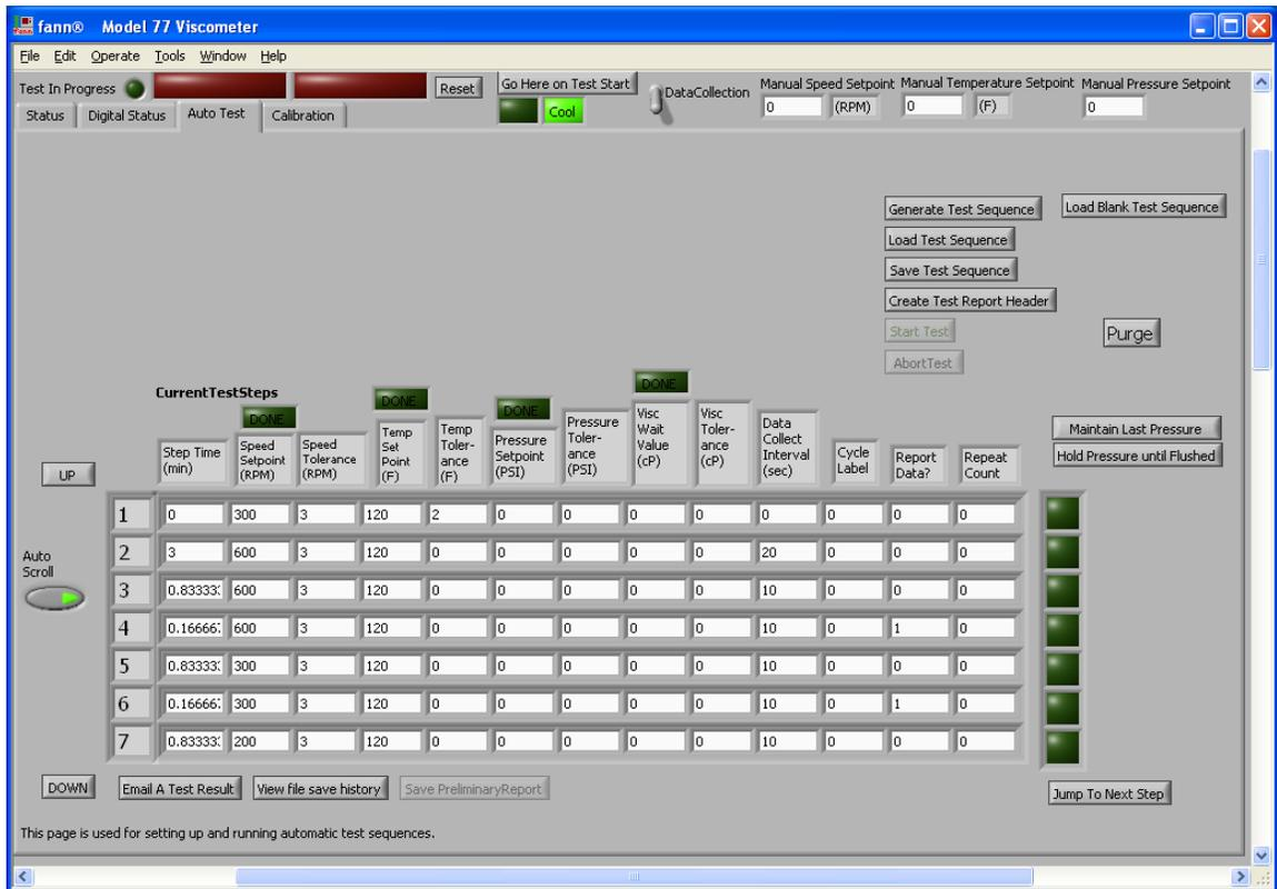
**Figure 5-29 Pressure set point is set to zero**
