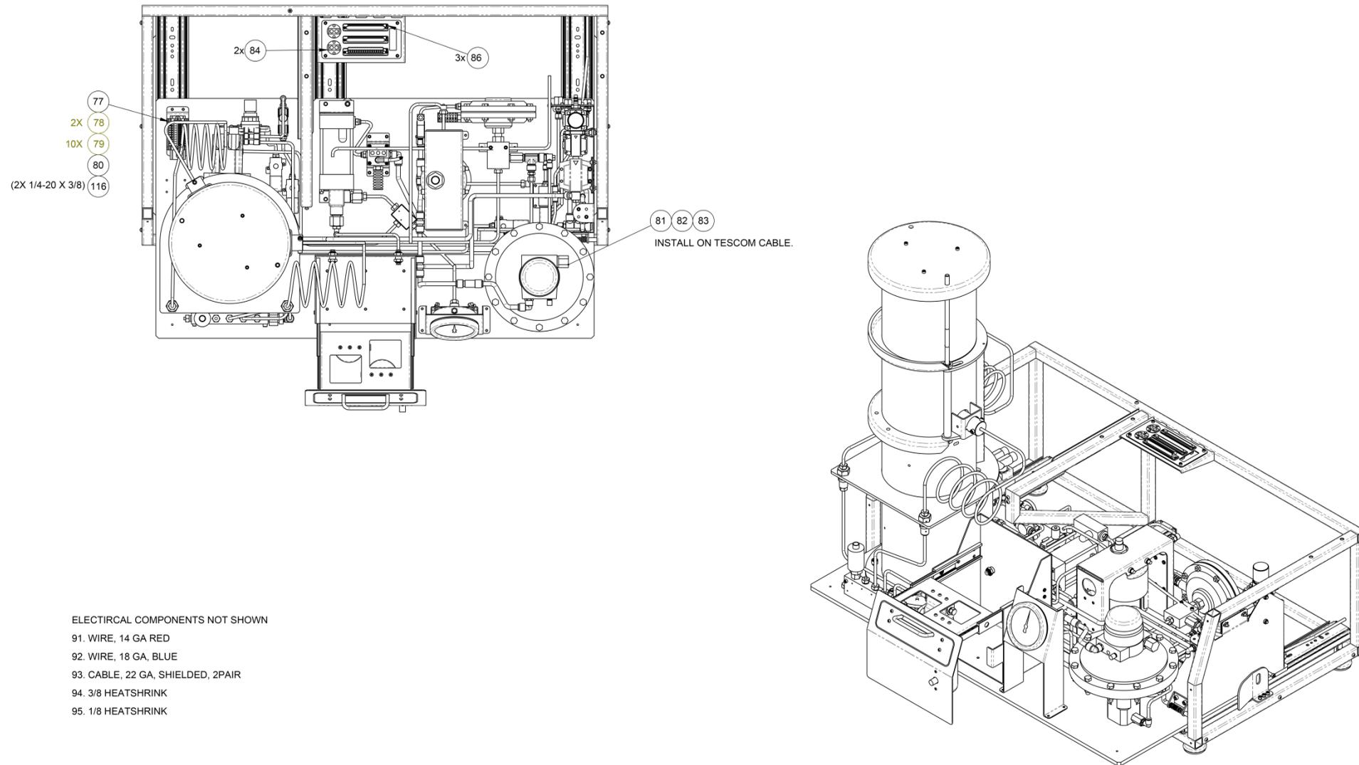
Figure 9-8 iX77 Mechanical, Electrical Components
