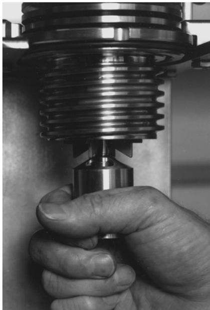
**Figure 5-31** Installing bob shaft assembly
