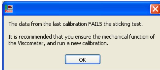
**Figure 5-1 Calibration failure dialog**
