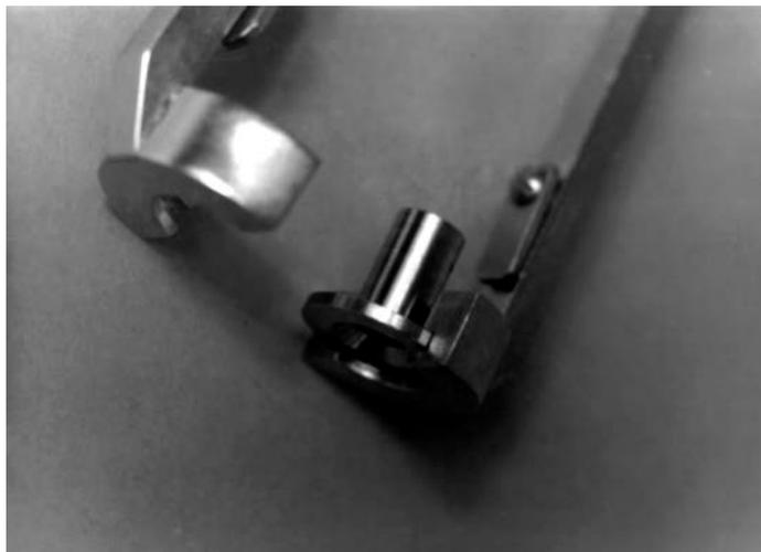
**Figure 5-57 The Pivot Bushing in the groove of the Puller**
