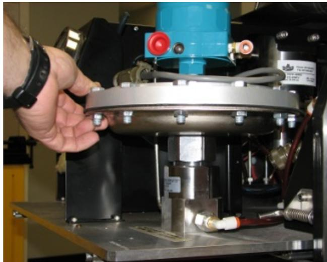
**Figure 7-9 Valve Disassembly**
