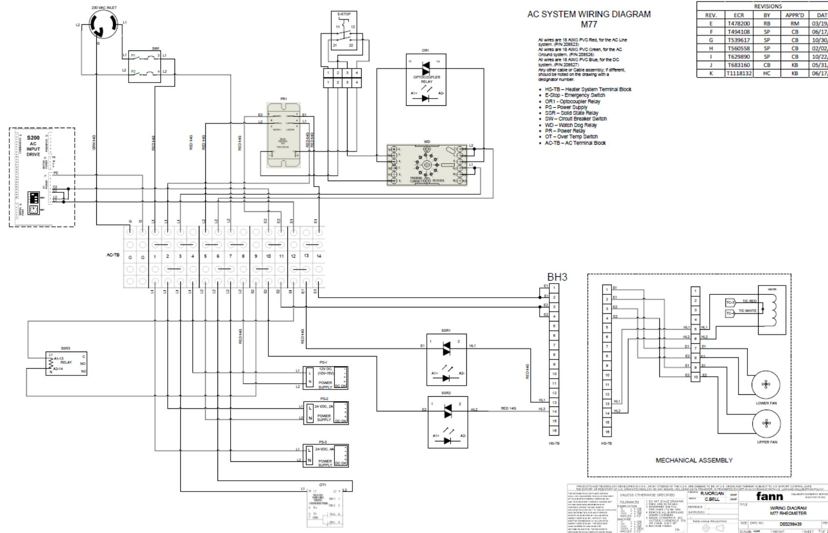
Figure 9-11 iX77 AC System Wiring Diagram
