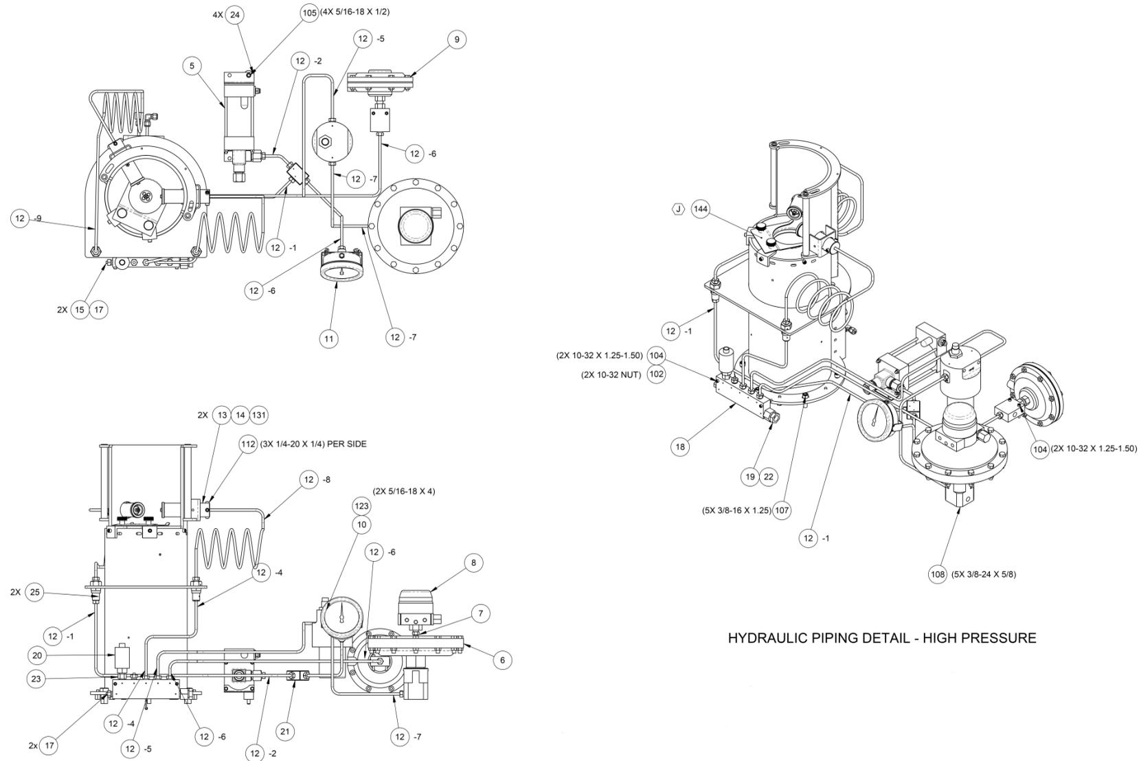
HYDRAULIC PIPING DETAIL - HIGH PRESSURE
