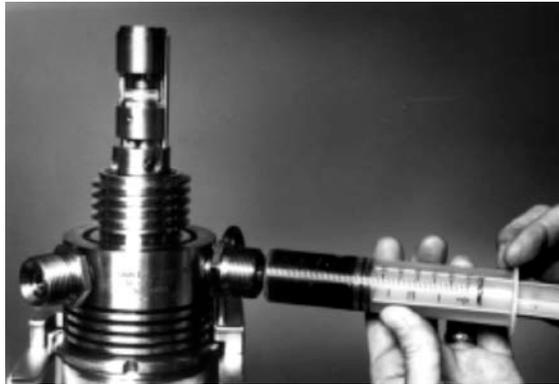
**Figure 5-41** Injecting the sample
