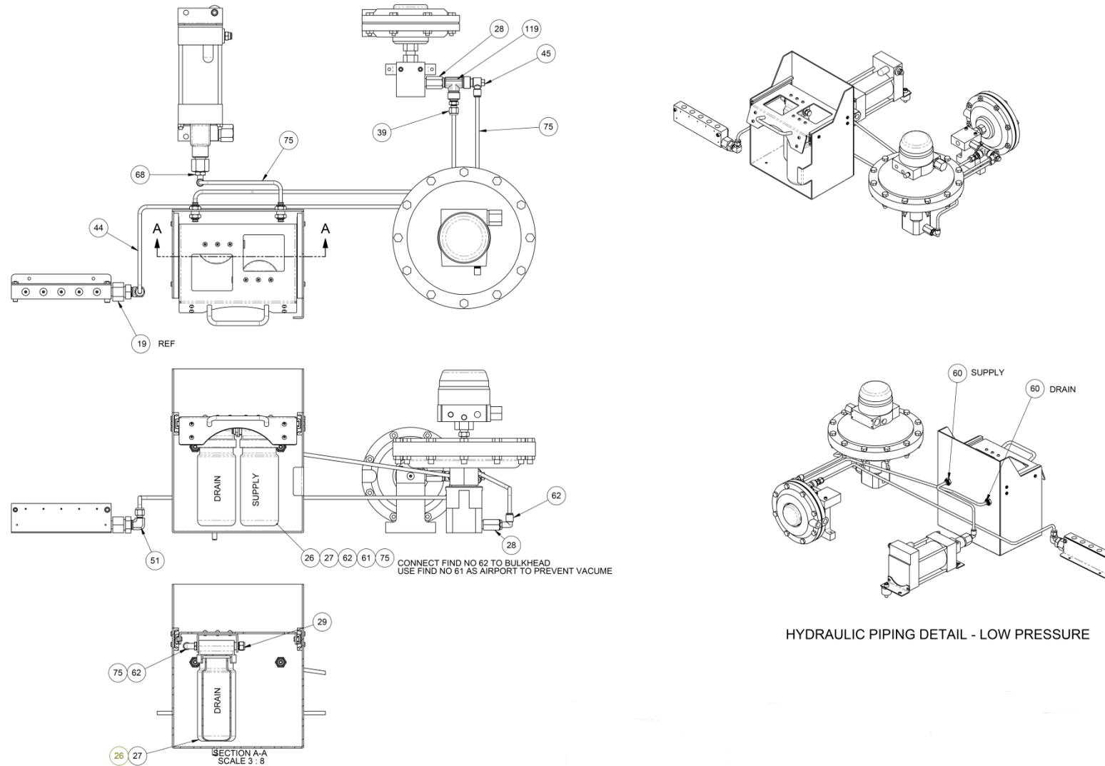
Figure 9-5 iX77 Mechanical, Hydraulic Piping, Low Pressure
