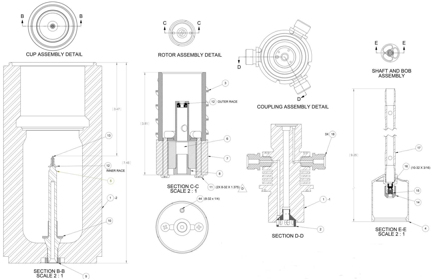
Figure 9-15 iX77 Cell Cup, Rotor, Coupling, Shaft & Bob
