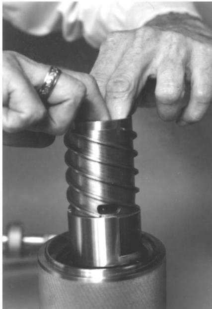
**Figure 5-32** Installing rotor in cell
