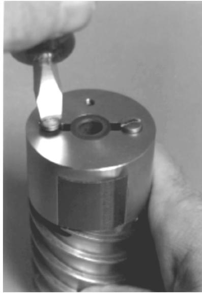
**Figure 5-44 Disassembling the rotor**
