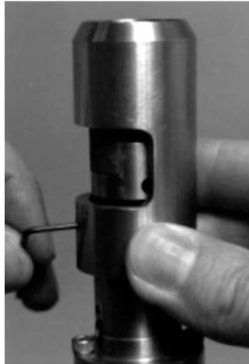
**Figure 5-60 Removing the pivot cap**
