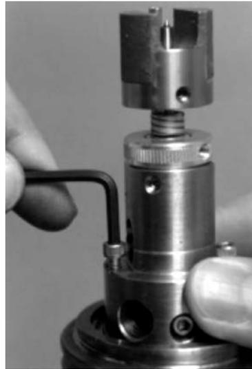
**Figure 5-46 Removing the torsion spring module**
