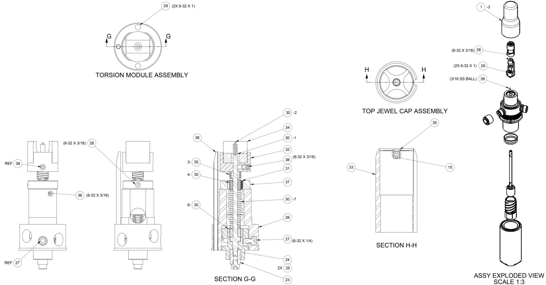
Figure 9-16 iX77 Torsion Module and Top Jewel Assemblies
