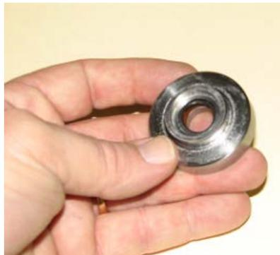
**Figure 7-20 O-ring and Backup Ring**
