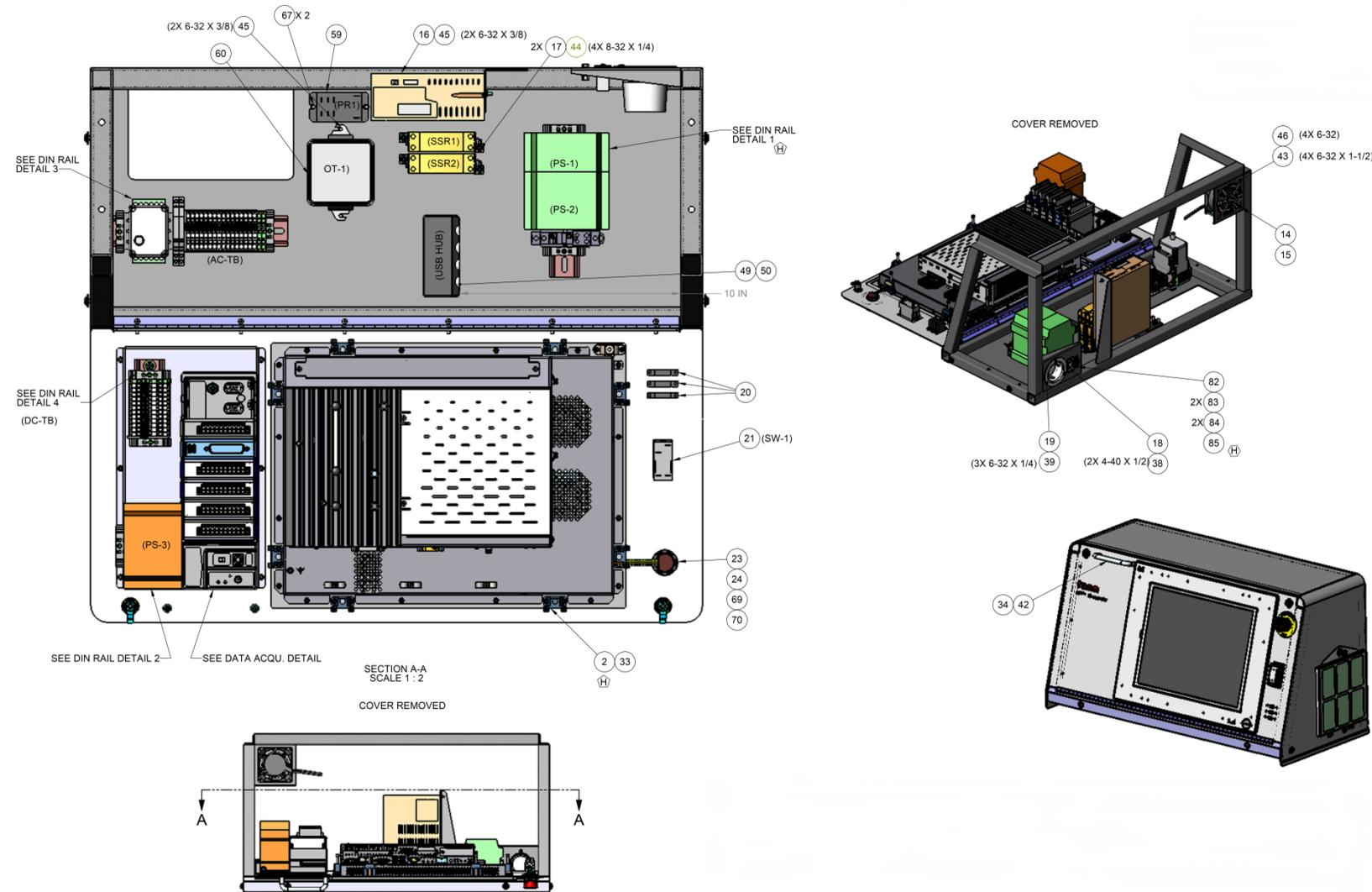
Figure 9-9 iX77 Electrical Assembly, Main Components
