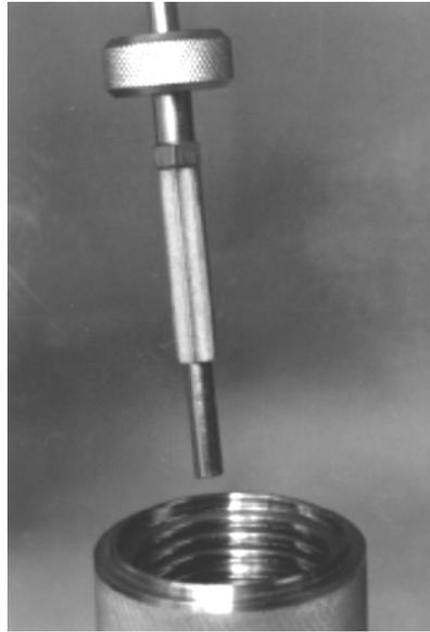
**Figure 5-53** Pushing the inner race onto the pivot
