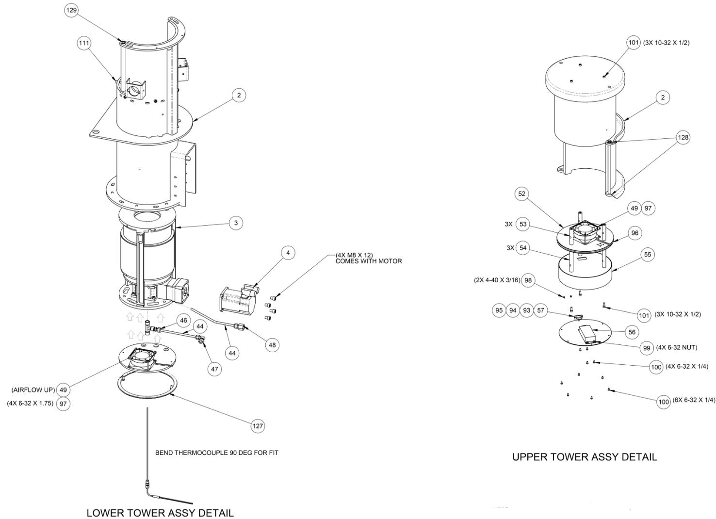
Figure 9-3 iX77 Mechanical, Tower Assembly
