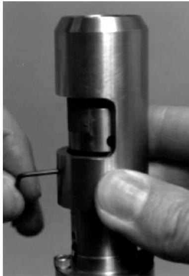
**Figure 5-62** Removing the pivot cap
