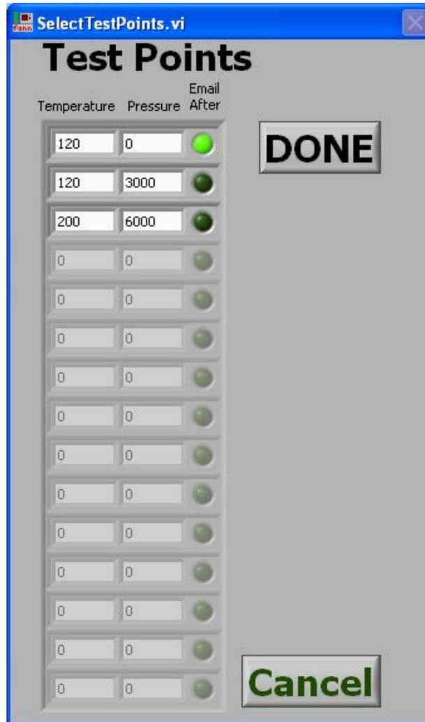
Figure 5-19 Fill in temperature and pressure test points
