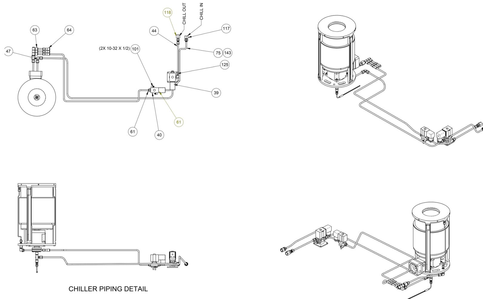
Figure 9-7 iX77 Mechanical, Chiller Piping
