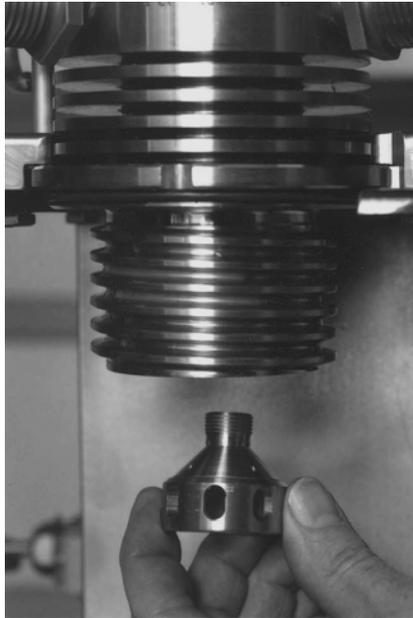
**Figure 5-30** Installing type “S” baffle
