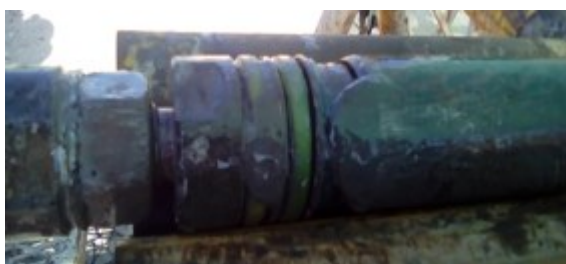
Figure 1. Core barrel back coated in drill solids. Fluid contains no QUIK-TROL GOLD, QUIKMUD GOLD or PENETROL DRY
