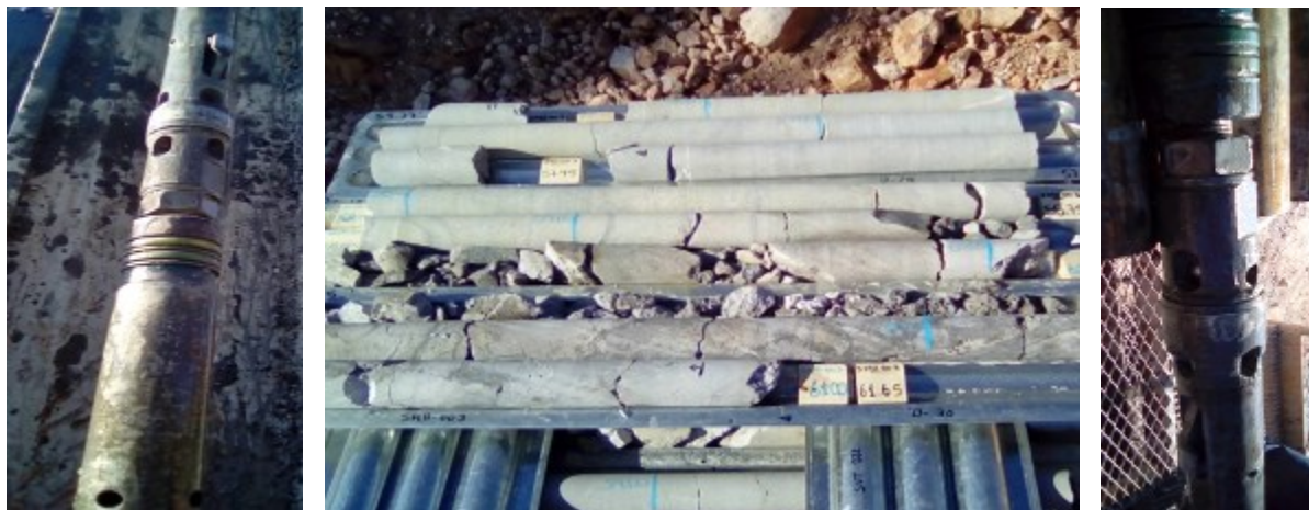
Figure 3. Examples of Clean Core Barrel Assembly Back Ends and Core showing no signs of excess sticky solids following addition of PENETROL DRY.
