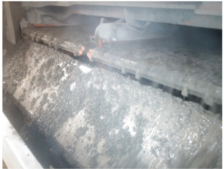
Figure 2. Drilled cuttings shown on shaker deck.
