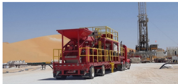
Mobile Vertical Cuttings Dryer system arriving at the rig site in Oman.
