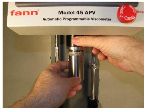
3. Level the system by adjusting the four corner feet and observing the bulls eye level (behind the top cover).
