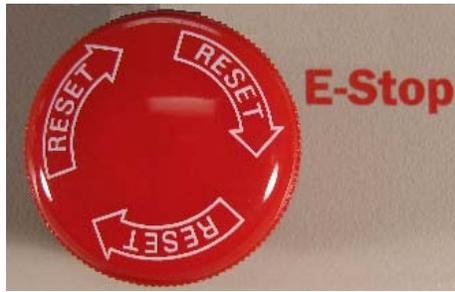
The **E-Stop** button (on front panel) can always be used to stop the drive motor.
