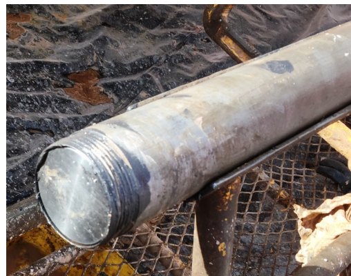
Figure 7. Piston at bottom of its stroke in Inner Tube
