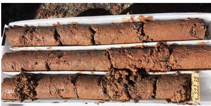
Figure 7. Core at 222m following two injections of FUSE-IT
