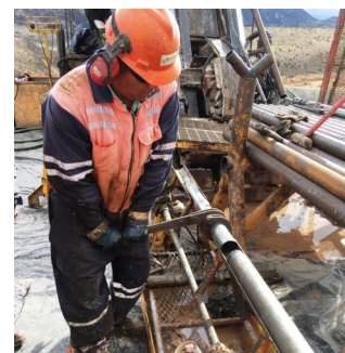
Figure 4. ROC Tool Assembly
