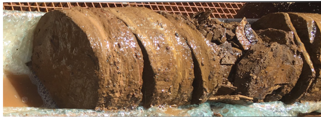
A recovered six inch core
