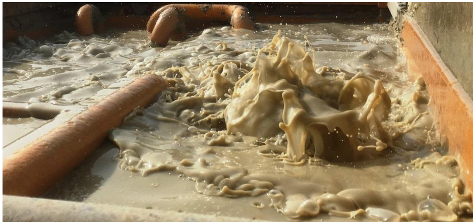
Figure 13. Low filtrate (8.5 ml/30min) lubrication fluid constructed from QUIK-GEL™ , QUIK-TROL® GOLD and FUSE-IT® additives
