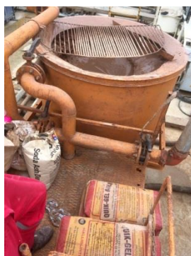
Figure 5. – Building lubrication fluid (left) – Addition of FUSE-IT in low concentration to reduce jacking force and skin friction (right)
