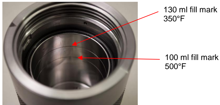
Figure 5-1 Cell showing fill marks inside
