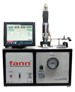
is equipped with state-of-the-art temperature control and data acquisition systems that provide ease of use for the operator. Temperature control is programmed through the use of a touch screen monitor. A plot showing temperature, pressure and consistency may be plotted on any printer or shared through the computer.
