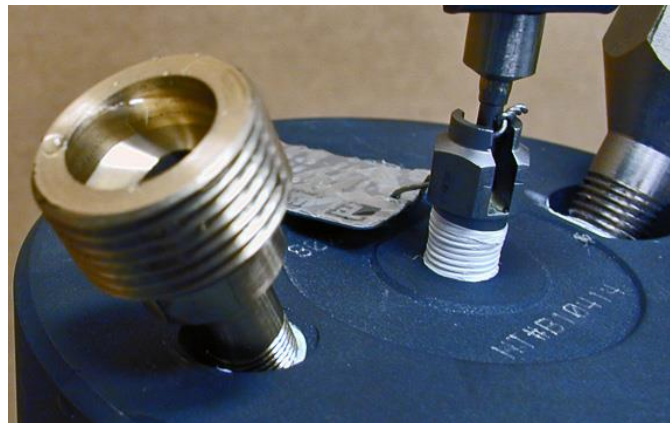
Figure 5-15 Water expelled as lid tightened
