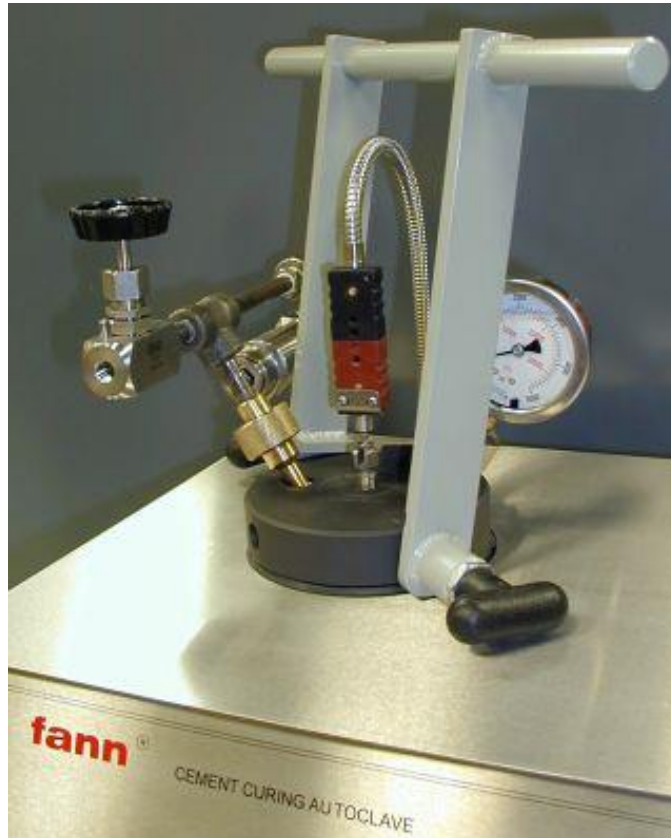
Figure 5-18 Place chamber into autoclave, remove handle
