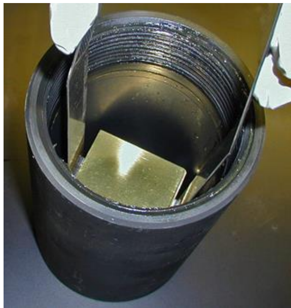
Figure 5-12 Lower mold into chamber – 2
