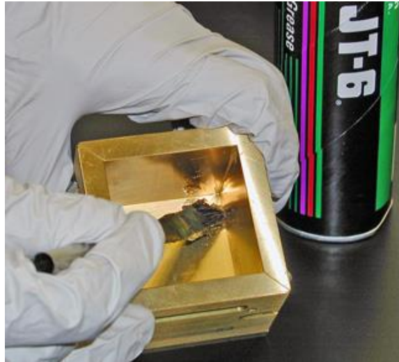
Figure 5-5 Grease mold interior
