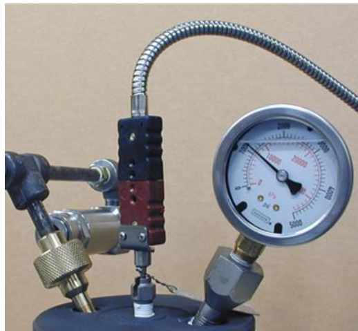
Figure 5-21 Set initial chamber pressure
