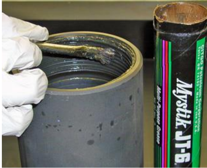
Figure 5-13 Grease chamber threads
