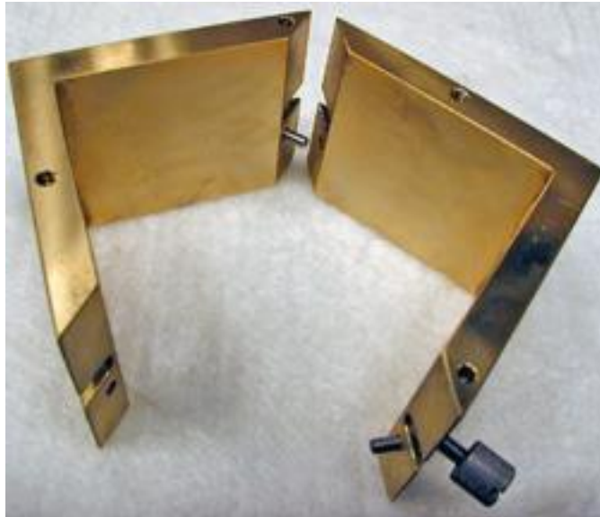
Figure 5-1 Pins align the mold halves
