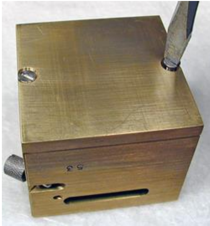
Figure 3-5 Cement Mold Base
