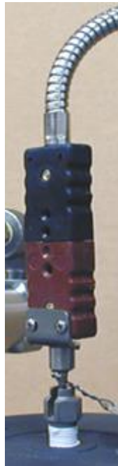
Figure 5-20 Connect thermocouple cable
