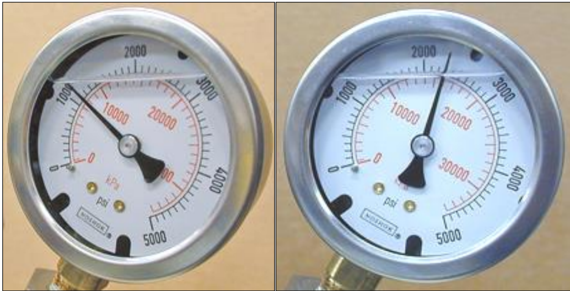
Figure 5-22 Initial pressure (left), increased pressure from temperature rise (right)
