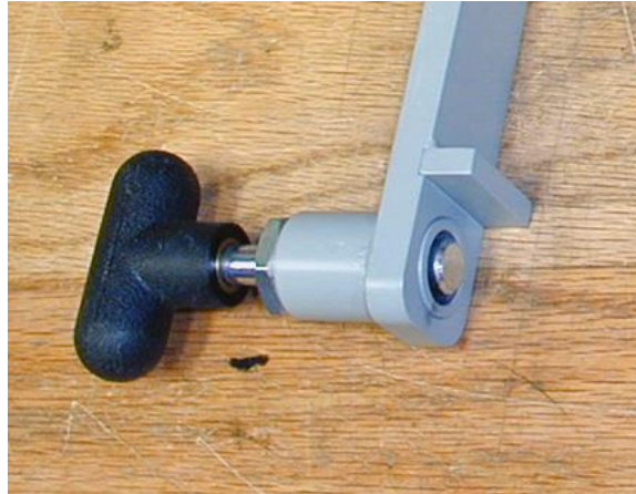
Figure 5-16 Handle spring loaded pin retracted
