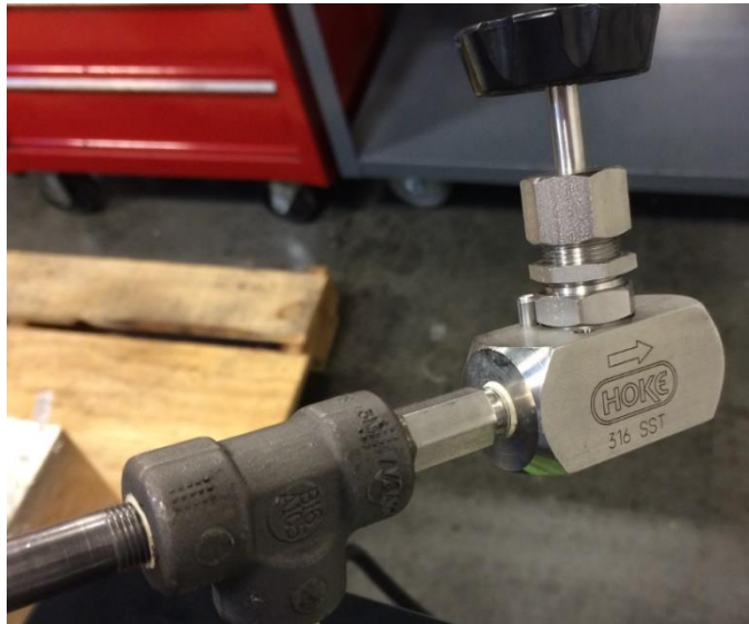
Figure 3-1 Manual Needle Valve and Pressure Relief Valve
