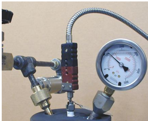
Figure 3-2 Pressure Manifold, Thermocouple, Pressure Gauge
