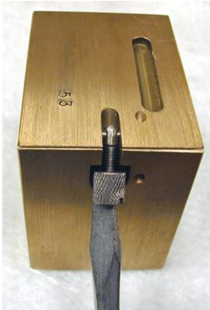
Figure 5-2 Clamps hold mold halves together
