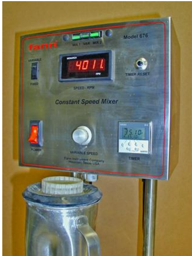
Figure 5-6 Mixing Cement Slurry
