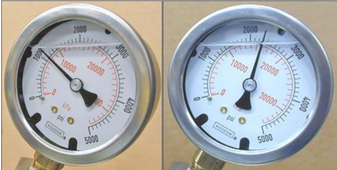
Figure 3-9 Initial pressure (left), increased pressure from temperature rise (right)
