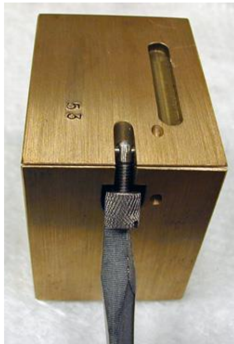
Figure 3-4 Cement Mold Clamp
