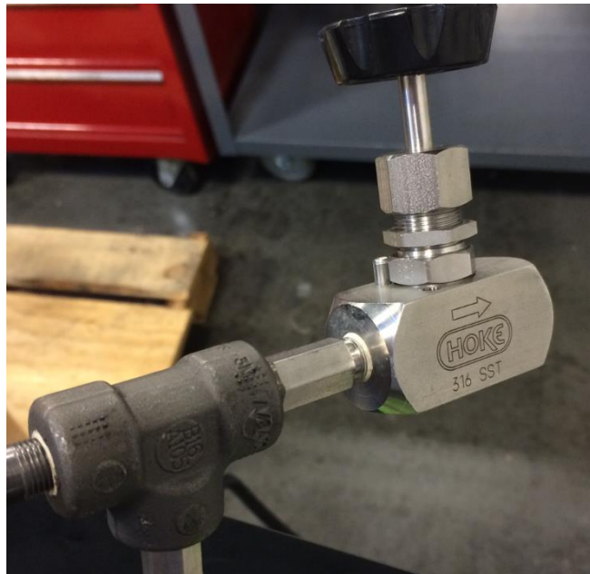
Figure 3-8 Pressure source connected to needle valve
