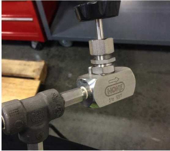
Figure 5-19 Attach valve and manifold
