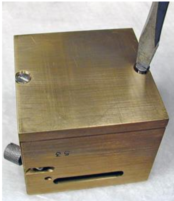
Figure 5-4 Tighten base plate to mold
