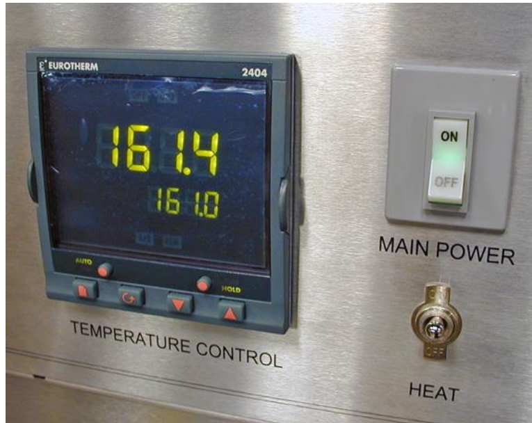
Figure 3-6 Temperature Controller, Main Power, Heat switch
