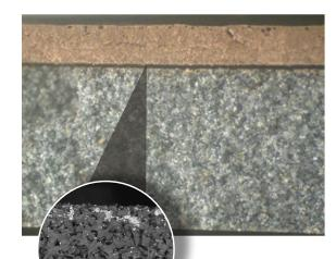
Here is a cross-section of a ceramic disc with filter cake and BaraFLC Nano-1 sealant under magnification. This shows how the nanoparticles pass through the cake and seal pore space.
