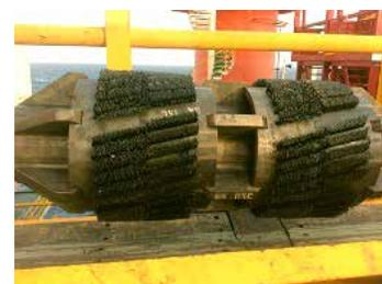
*This brush is residue-free after application of an engineered cleanout spacer containing BaraKlean<sup>®</sup>-648 casing cleaner.*
