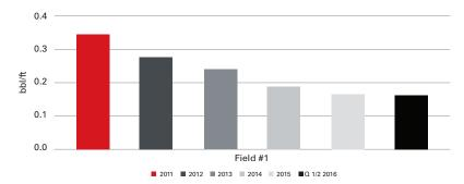
Non-aqueous fluid (NAF) losses were cut by over 50 percent in a six-year comparison, down to less than 0.2 bbl per foot drilled.
