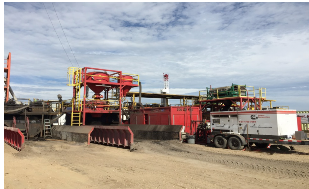
The BaraG-Force™ VacVCD configuration features a small footprint. Wet cuttings are delivered from the shakers to the hopper via the pneumatic vacuum line. A rotary feed valve below the hopper minimizes buildup, and recovered drilling fluid is pumped to an integrated catch tank. Dried cuttings are ejected below the dryer for easy removal. An auxiliary site response pod to assist with spills and cleanups is connected at the right of the hopper.
