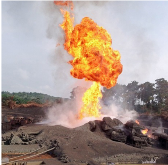
Figure 1. The catastrophic blowout of the shallow gas well created a crater that swallowed up the rig and caused the drillstring to drop down the open hole.
