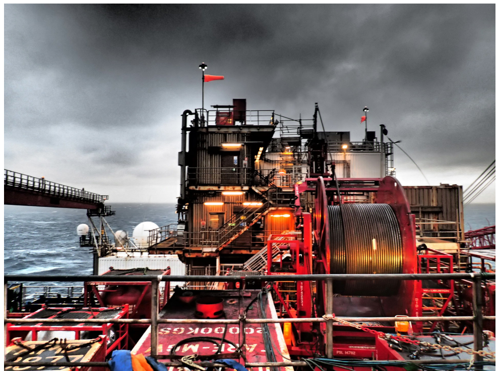
Coiled-tubing placement of reservoir barriers was proven for North Sea applications on the project.
