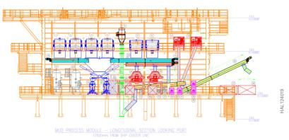
Flow path from shakers (upper left) via augers to cuttings dryers. Centrifuges installed on pits (upper right) with discharge via auger to cuttings catch box.
