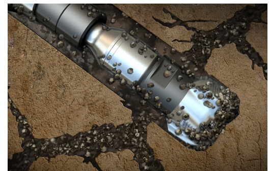
The BaraShale™ Lite direct emulsion fluid system is designed to prevent lost circulation and washout while minimizing dilution and waste volumes.
