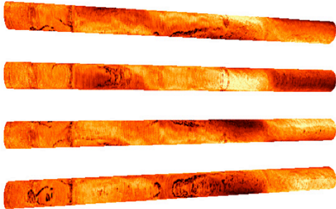
These illustrations include log examples showing high-resolution ultrasonic interpretation. The top image depicts fracture interpretation from high-resolution reflection amplitude images in the Rodessa Limestone formation. The middle image shows high-angle bedding features seen on both reflection amplitude and radius images within the Rodessa Limestone formation with a borehole inclination of 87 degrees. The dark feature seen between 3,753 feet and 3,754 feet on all the images is caused by the kick pad from the mud motor at the start of a slide section. The bottom image shows 3D visualization of high-angle bedding features.
