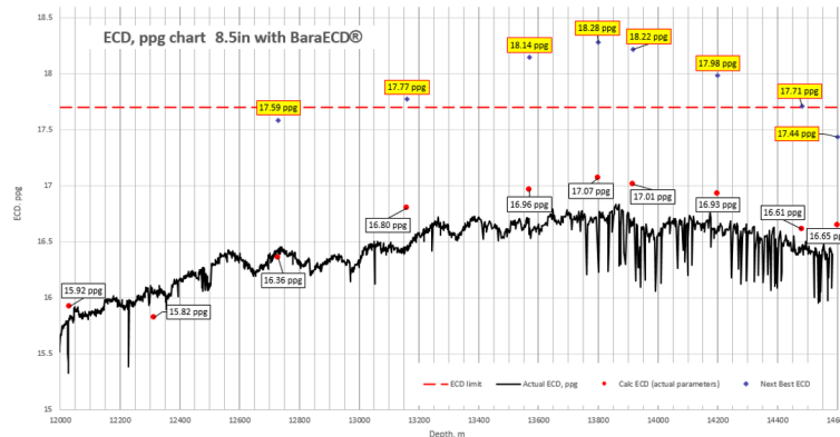
This chart highlights BaraECD performance by mapping the DFG modeled ECD (red dots) over the actual (PWD measured) ECD. The purple crosses are the modeled ECD expected from the next best NAF.
