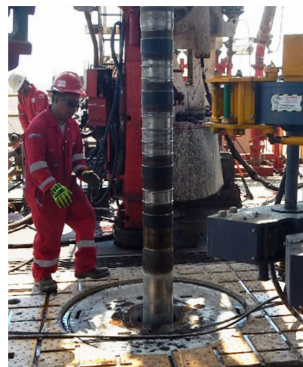
XtremeGrip® liner hanger on rig floor prior to running in hole
