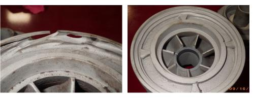
Left » Erosion was significant in standard style diffusers. Right » Diffuser with Erosion Buster® design shown fully intact.
