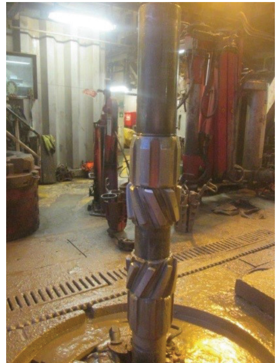
Well No. 2 – A 9 5/8-in. Drill Tech® scraper condition after drilling 341 meters (1,119 feet) of open hole
