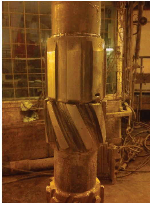
Well No. 1 – A 9 5/8-in. Drill Tech® scraper after drilling tieback, shoe track, and 81 meters (266 feet) of open hole
