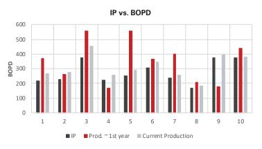
Comparison of the increase in oil production value within a year of production after the N-FLOW<sup>™</sup> 325 system was applied in the giant heavy oil Boscán field, along with a current measurement over the following 2–3 years.
