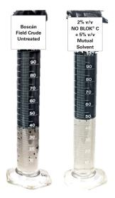
*Oil/completion brine compatibility test after 24 hr of static aging. Without proper proactive treatment, drilling fluid filtrate, crude oil and brine can all create emulsions when they mix.*
