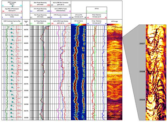
Quad-Combo Service and AFR<sup>™</sup> solution delivers critical formation evaluation data with wireline quality high-resolution images, saving costs and time in a horizontal well.
