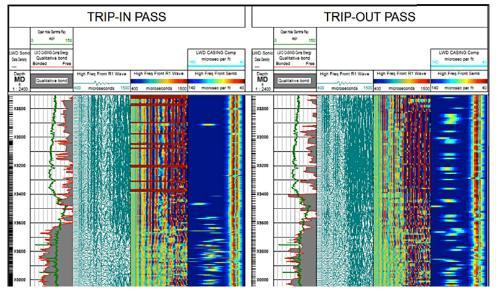
TOC analysis performed inside 7%-inch casing during the trip-in pass of a cement cleanout run (left) compared to the trip-out pass (right). The trip-out pass occurred with lighter mud than the trip-in pass, following displacement of the drilling fluid.
