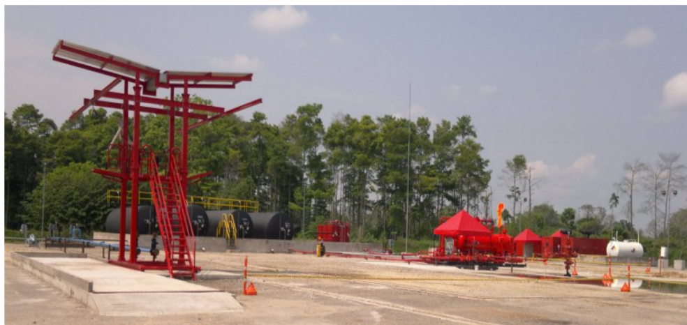
Photo of standalone Aullador-1 EPF, showing its modular layout and, at left, a truck loader structure
