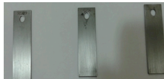
Figure 1. Corrosion test conducted over 14 days at 400°F (204°C). Coupon 1, control; Coupon 2, treatment with 1% by volume BARACOR® 100 corrosion inhibitor; and Coupon 3, treatment with 2% by volume BARACOR 100 corrosion inhibitor.
