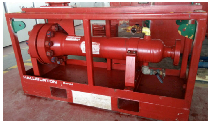
Figure 3. A Halliburton HT Shearing Unit was rigged up to the rig pumps and the fluid was sheared offline at 2,000–3,000 psi while mixing the fluid components.
