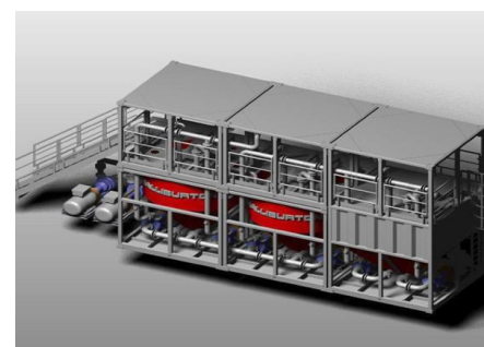
Cuttings reinjection slurrification system
